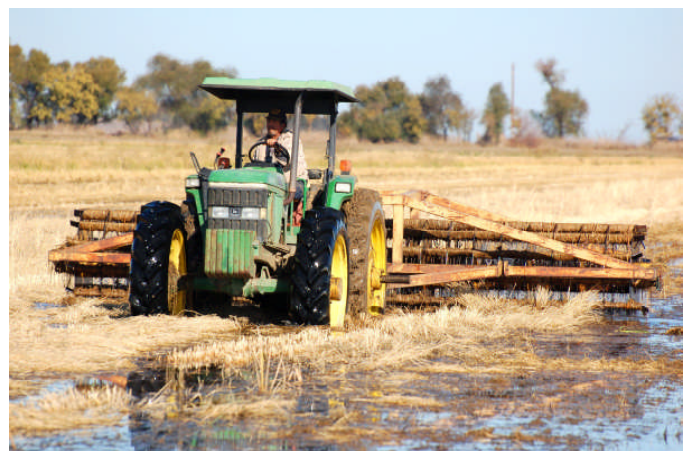
Rice Residue Management with a rice straw roller, near Winters CA. Photo - Phil Hogan, District Conservationist, Woodland
