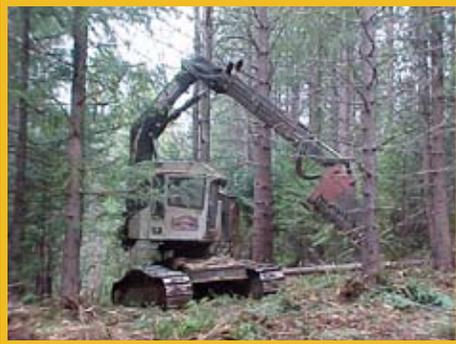
*Mastication equipment destroys brush undergrowth, removing ladder fuels. Photo by NRCS.*
